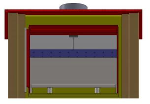
REPEAT THE PROCESS TO INSTALL THE RIGHT HAND SIDE BAFFLE PLATE. PULL BOTH BAFFLE PLATE FORWARD AS FAR AS POSSIBLE. ENSURE THAT BOTH BAFFLE PLATES ARE CENTRED. THIS WILL ENSURE A GAP ON BOTH SIDES.
