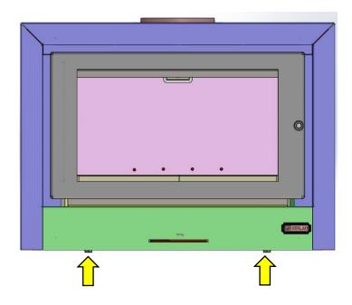
NOTE:- When installing this unit onto a table, make sure to leave the 4x bolts in place. The bolts are necessary to allow air flow to the underside of the firebox. The removal of these bolts will lead to overheating to the underside of the unit and eventually cause malfunction. The removal of these bolts could void your warranty.
