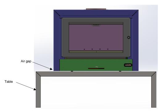
There must be an air gap between the bottom of the appliance and the top of a table. This is necessary to allow air flow to the appliance.
