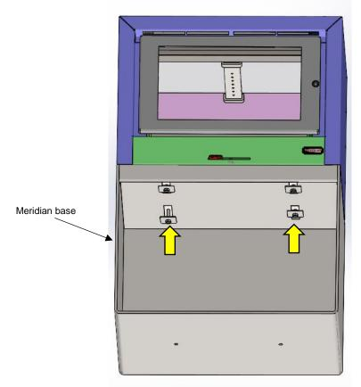
The bolts will need to be removed when the appliance is installed onto a meridian base. However, the same bolts must be used to fix appliance to the meridian base.
