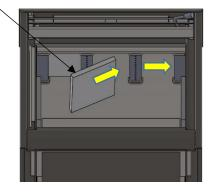
3. REPEAT STEP 2 PROCESS BUT THIS TIME MAKE SURE THE BAFFLE PLATE 2 SLIDES OVER BAFFLE PLATE 1.
